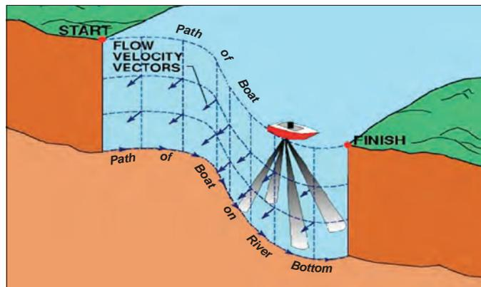
**Figure 6.** Acoustic Doppler Current Profiler (ADCP) mounted in a small watercraft, is used for measuring the discharge of a river. The ADCP acoustic beams are directed down into the water as it is guided across a river channel.
