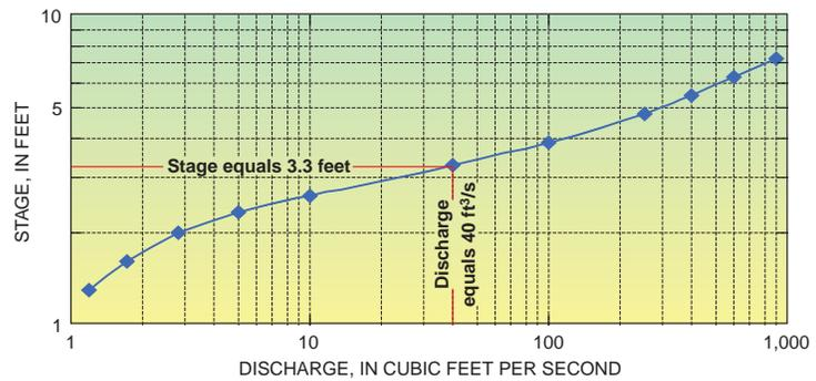
**Figure 8.** Example of a typical stage-discharge relation; here, the discharge of the river is 40 cubic feet per second ( $\text{ft}^3/\text{s}$ ) when the stage is 3.30 feet (ft). The dots on the curve represent concurrent measurement of stage and discharge.
