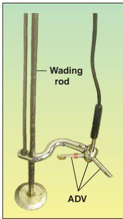
**Figure 7.** Acoustic Doppler Velocimeter (ADV) mounted on a wading rod.
