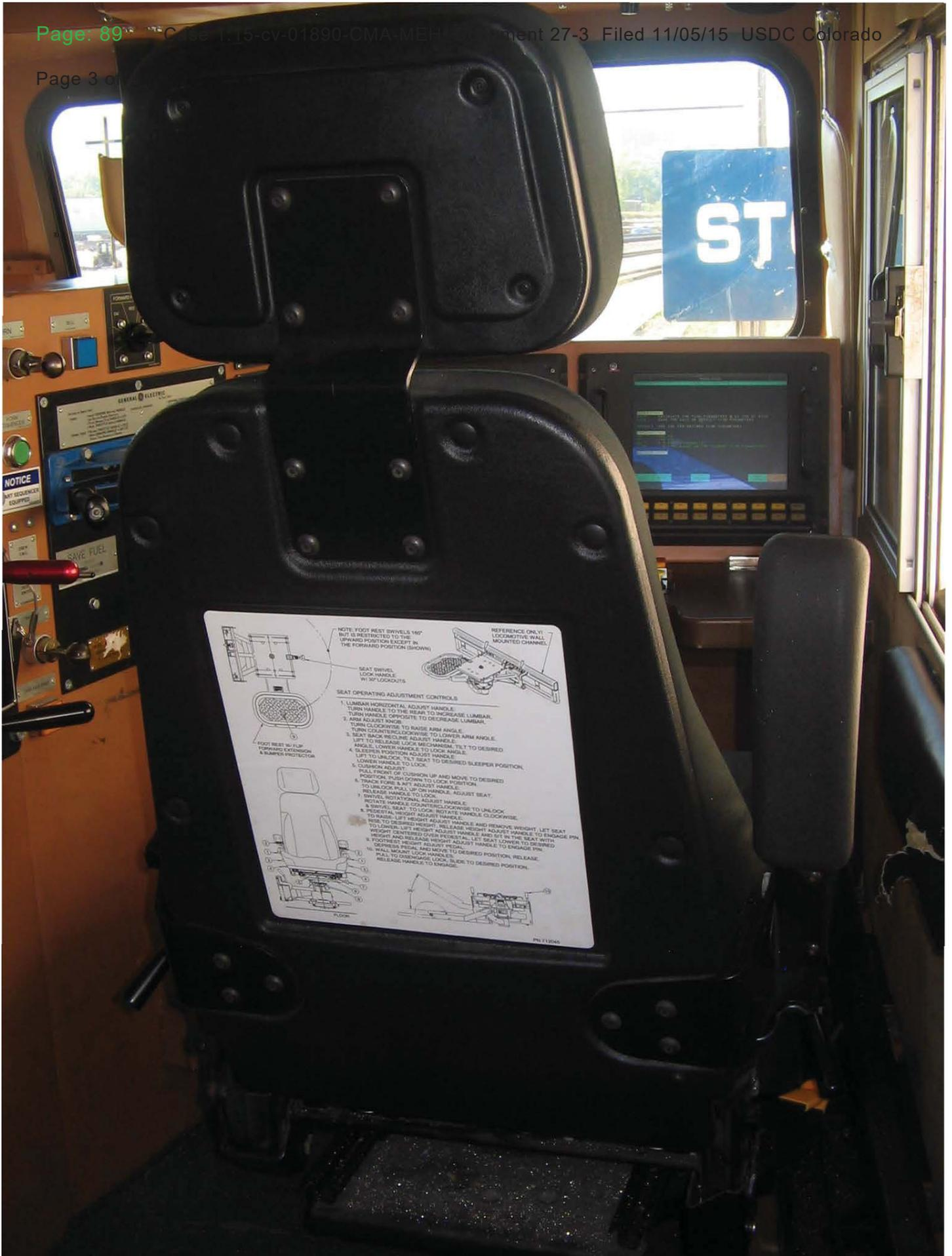
NOTE: FOOT REST SWIVELS 140° BUT IS RESTRICTED TO THE UPWARD POSITION EXCEPT IN THE FORWARD POSITION (SHOWN)
